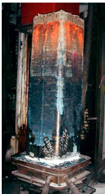
Figure 3 Appearance of ASR ingot of steel 19CrMnNi, 560 × 560 mm, 4 t.
