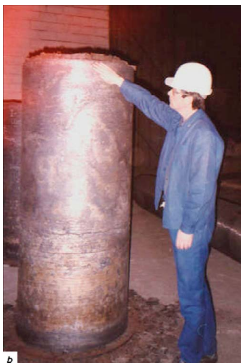
Figure 5 Appearance of ASR ingots of steel CrMn18.18 , 560 × 560 mm, 3 t (a) and 860 mm dia., 1900 mm height, 8 t (b).
