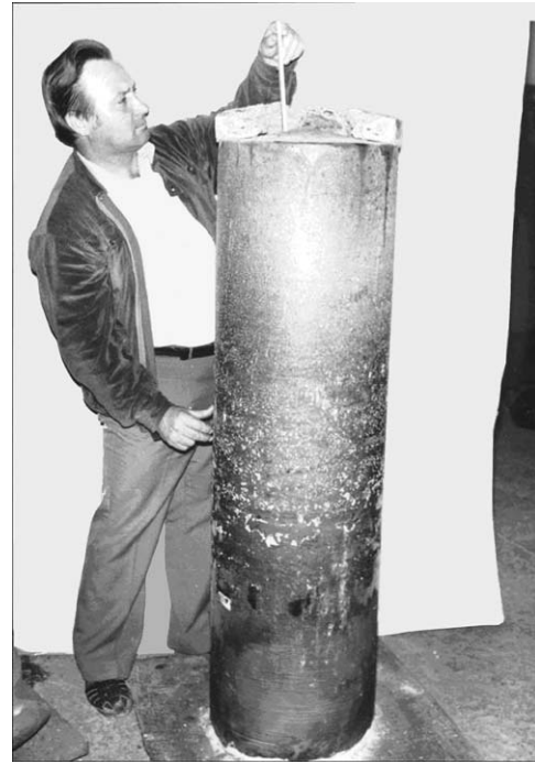
Figure 7 Appearance of ASR ingot of steel, 38CrNiMoV1.3 400 mm diameter and 1500 mm height.
