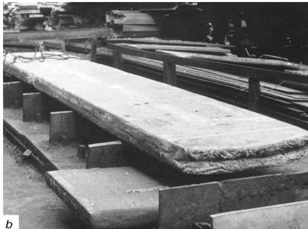
Figure 6 Appearance of ASR slag ingot of titanium VT1-0. 650 × 1150 mm section, 1700 mm height and 5 t mass (a) and 115 mm thick plate, rolled from it (b)
